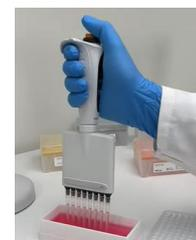
How to Use Picus® 2 Electronic Pipette – Pipetting Mode With Repeating Blowout and Mixing
