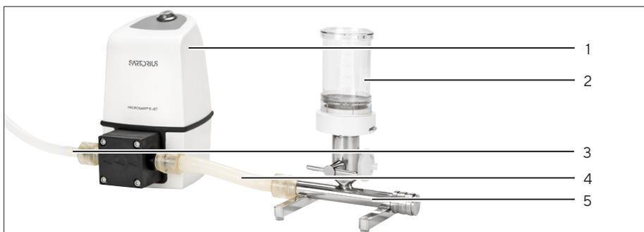
Fig. 5: Process structure for the filtration (in this example, Microsart® 1-way manifold with Biosart® 100)
